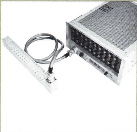
WJ-136 Multi-channel, double-tuned YIG filter; individual electronic tuning of the 20 channels permits varying its bandpass characteristic
